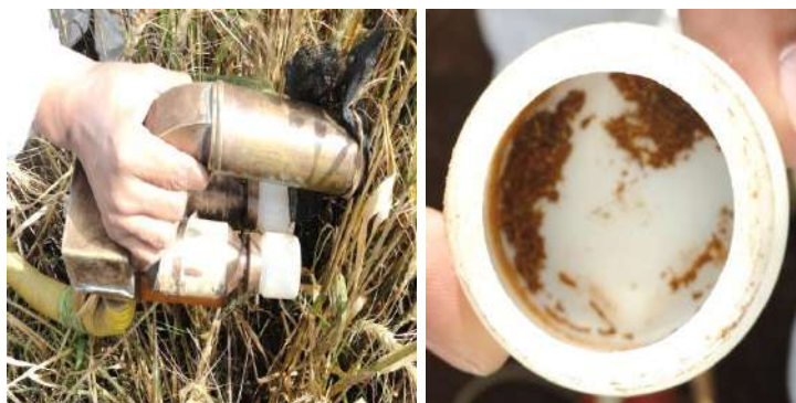
Fig. 14. Cyclone collector for rust inoculum in field & spore collected
