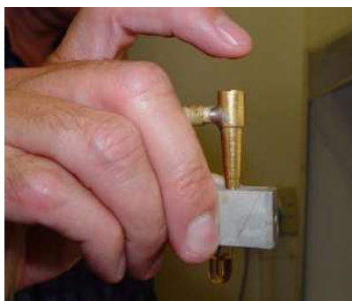
Fig. 21. Spray inoculation with hand atomizer and pressure pack inoculation
