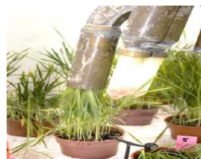
Fig. 13. Cyclone collector for rust inoculum in glasshouse
